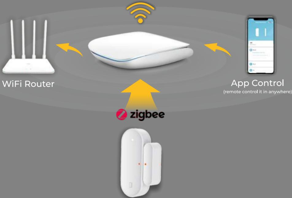
The Door sensor is connected through the Zigbee hub.
